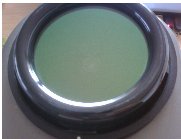
Measurement electrode with minor scratch from the test object, which does not affect the quality of captured GDV images
