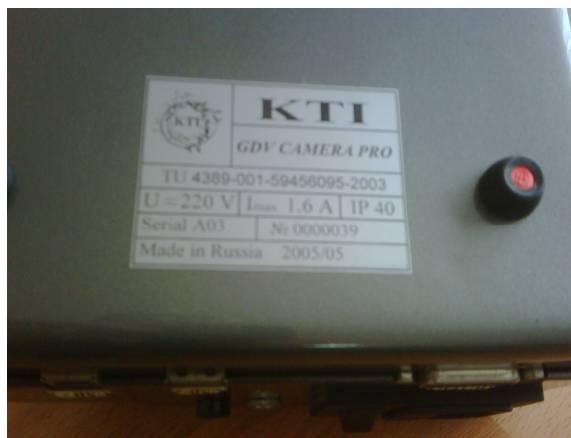
Identification plate, intact sealing of housing
